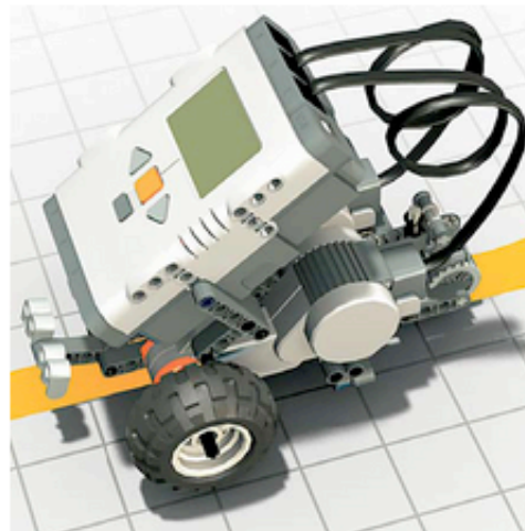
Figure 1 The 9797 LEGO car with two motors.
