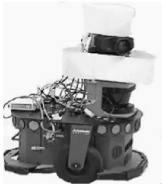
Fig. 4. A robot with laser and panned camera, the lens peering out through the hole in the color helmet.
