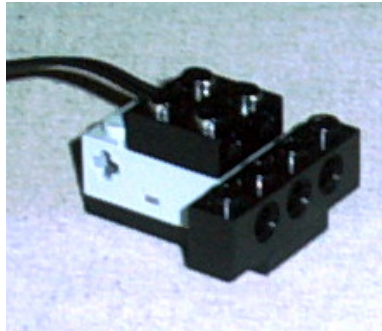
Figure 6: The simple sensor fitted with a LEGO brick to decrease the influence of ambient light.
